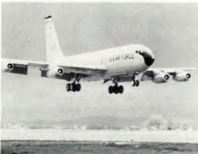
tle against corrosion, the C-135 will be repainted the same color as the nose of an F-16, duck-egg blue. Gloss paint would be much more effective against corrosion, but for tactical reasons, the paint will be flat.
